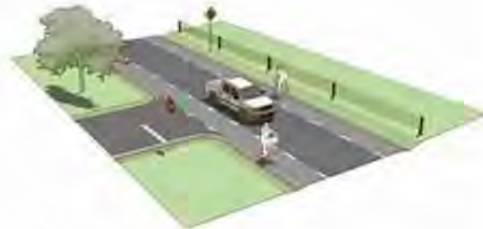
Figure 1. Schematic of an edge lane road.
