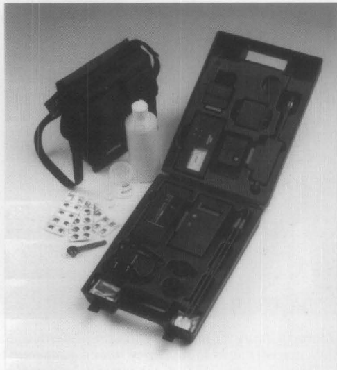
Fig. 14. Using instruments in this damp-check kit can help determine the relative change in wet conditions over time. This involves readings of air temperature, computing dewpoint temperatures, and tracking the moisture content of materials to indicate if they are drying properly. Photo: Dell Corporation.
