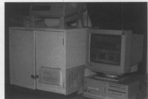
H. New computers tie a variety of monitoring and security features into a comprehensive system which provides warning and backup alerts when any of the system components are not functioning properly. Photo: © Isabella Stewart Gardner Museum, Boston.
